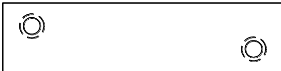
S-1 Special 14 Gauge 3/4" X 3" 3/16" Staggered Holes w/ CS
